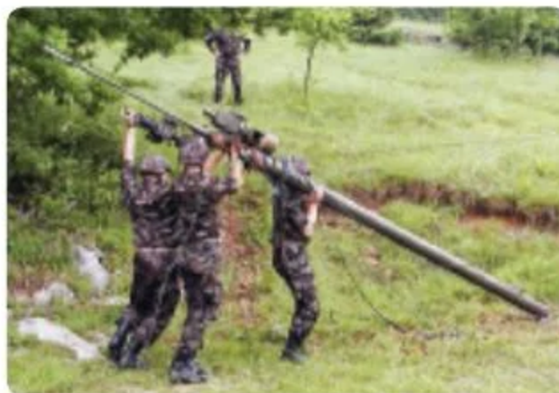
Deployment of lightweight telescopic EXL-mast
